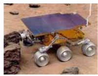
The Mars Pathfinder actually landed on the surface of Mars (in an inflatable 'ball') and deployed a 'roving vehicle' called Sojourner. Sojourner (see picture left) moved over the surface of Mars, taking pictures and information on the planet's surface and sending them back to Earth.
